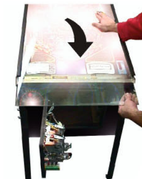
13. Open the Coin Door and pull the YELLOW HANDLE to the LEFT and at the same time pull up on the FRONT TOP MOLDING and remove. The GLASS can now be pulled out towards you and removed. TAKE CARE while moving; set glass on a safe surface.
