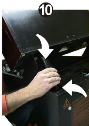
10. Lift the Backbox into the UPRIGHT POSITION (Ensure the cables do not get pinched).
