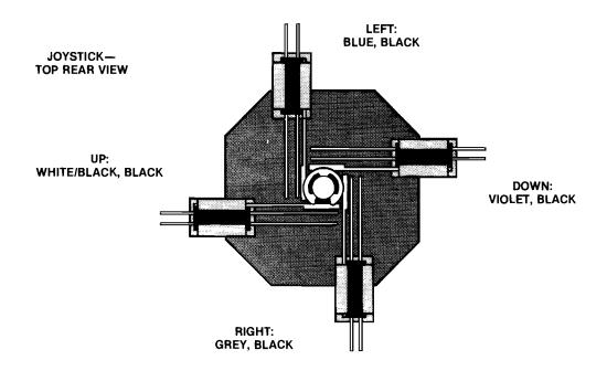
Figure 3-4 8-Position Joystick Assembly, continued
