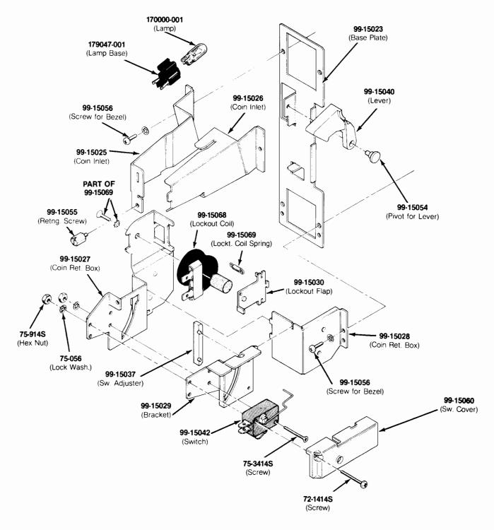
Figure 3-7 Vertically Mounted Coin Door A037619-xx C
