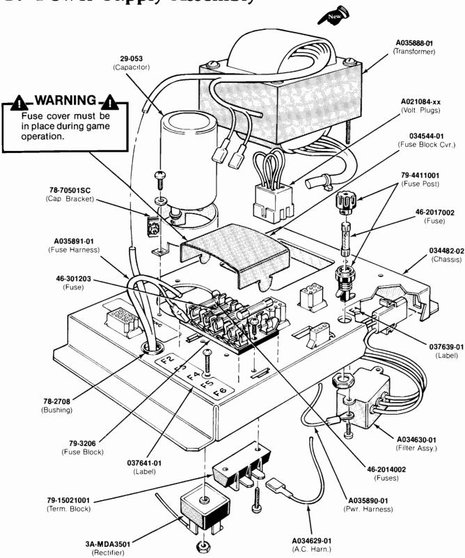
Figure 3-12 Power Supply Assembly A037671-01 and -02 C
