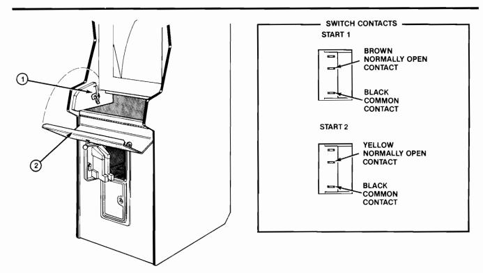
Figure 3-2 The Control Panel
