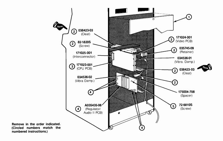
Figure 3-8 Printed-Circuit Board Removal
