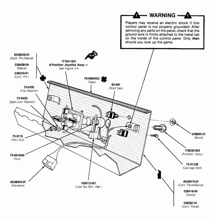
Figure 3-3 Control Panel Assembly Upright Cabinet A038414-01 A Ireland-Built Cabinet A038434-01 A
