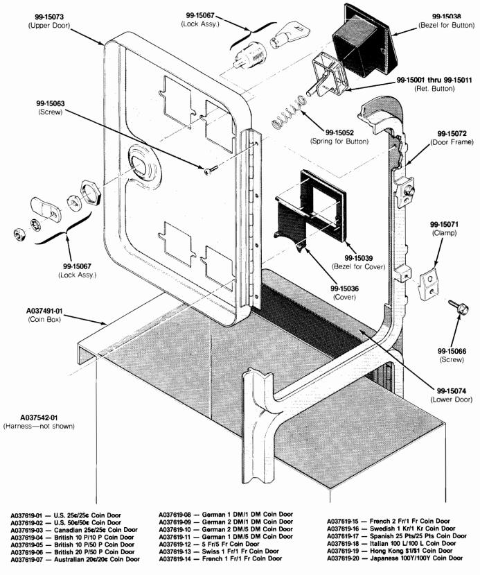
Figure 3-7 Vertically Mounted Coin Door, continued A037619-xx C
