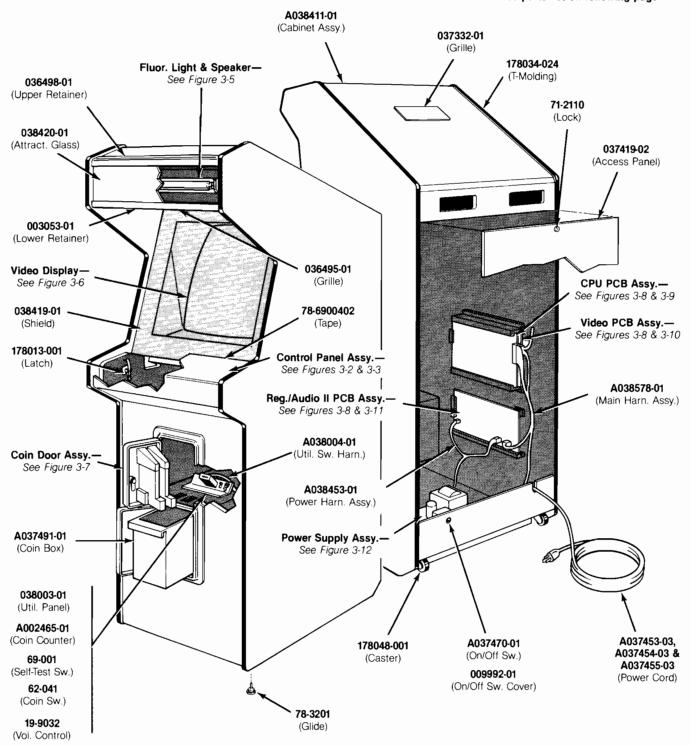
Figure 3-1 Cabinet-Mounted Assemblies Upright Cabinet A038410-01 A
