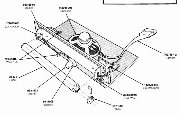
Figure 3-5 Fluorescent Tube and Speaker, continued Upright Cabinet Assembly A037417-01 and -02 G
