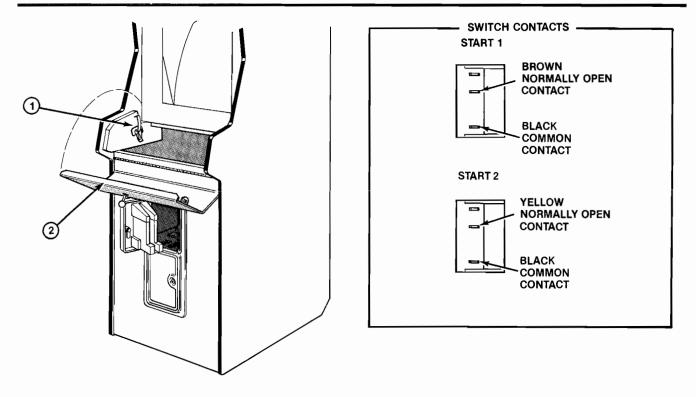
Figure 3-2 The Control Panel
