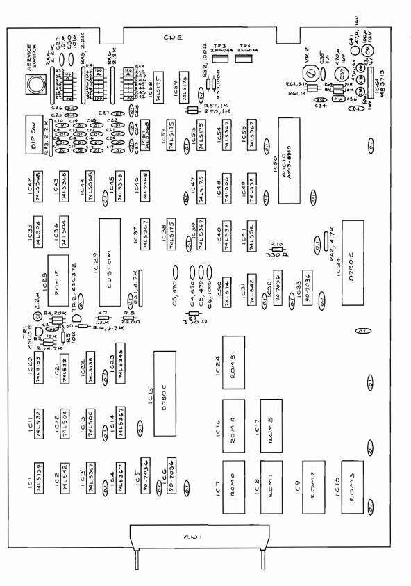
Figure 3-9 Kangaroo<sup>™</sup> Central Processing Unit PCB Assembly 171023-001
