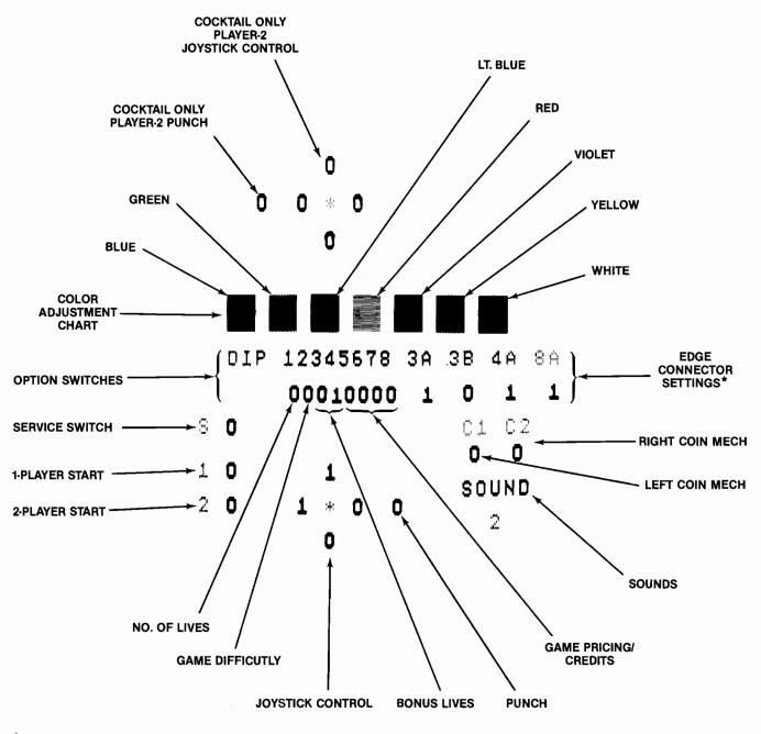
\* These represent harness connections on the CPU PCB. 1 means the pin is shorted to ground in the harness. 0 means there is no connection in the harness.
