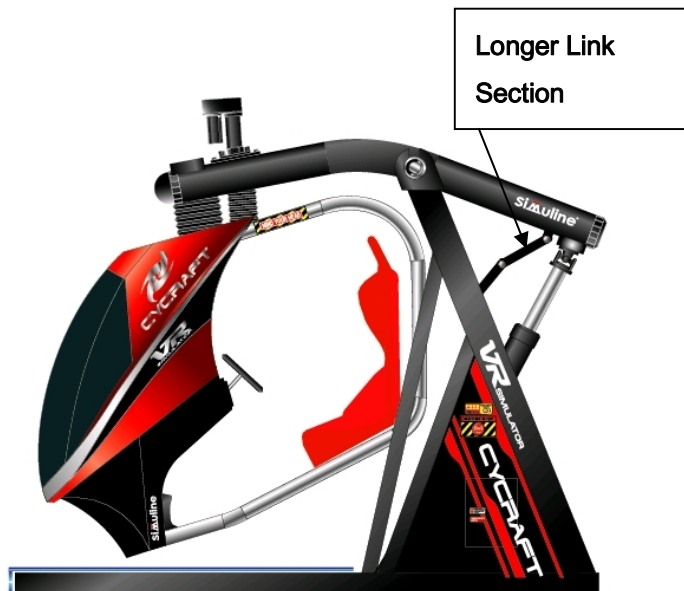
Figure of Cyrcraft after assembling the heave actuator and safety link
