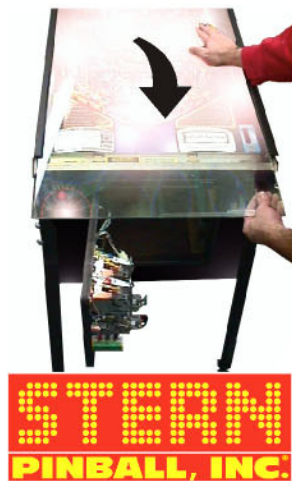
13. Open the Coin Door and pull the YELLOW HANDLE to the LEFT and at the same time pull up on the FRONT TOP MOLDING and remove. The GLASS can now be pulled out towards you and removed. TAKE CARE while moving; set glass on a safe surface.
