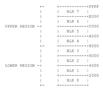
Each block can be programmed to be "mapped", or "non-mapped" via bits in the mapper's "mask" registers. NON-MAPPED means, simply, address out equals address in. Therefore, there are still only 64K bytes of non-mapped memory. MAPPED means that address out equals address in plus some offset. The offset is programmed via the mapper's "offset" registers.
