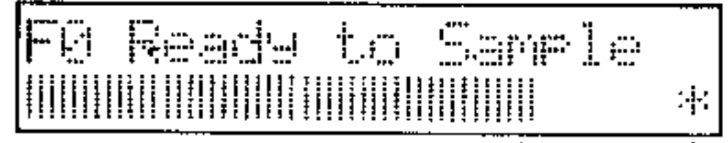
↑ Input signal level indication. ↑ Trigger level indication.
