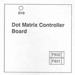
Dot Matrix Controller Board D10, +5V Circuit, Normallly On
