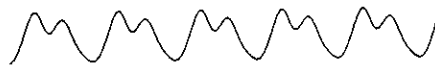
Reverberation wave of an electric Piano 1.5 second after the attack When the reverberations calm down, wave-forms become gentle.
