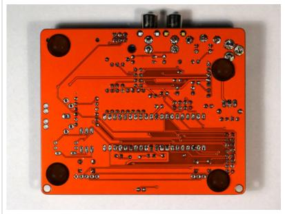
Place the 4 rubber bumpers as pictured. It's important to have them in place to help soldering the SNES connectors.
