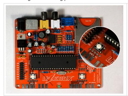
Add the *ISP* connector (notch goes inside) and the extension header (the grey side of the header is to be soldered).
