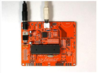
Insert **MCU** (ATmega644) into the DIP-40 socket. Notice one end of the chip has a notch, it goes the same way as the socket.
