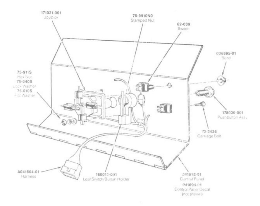
Figure 5-3 Control Panel Assembly
