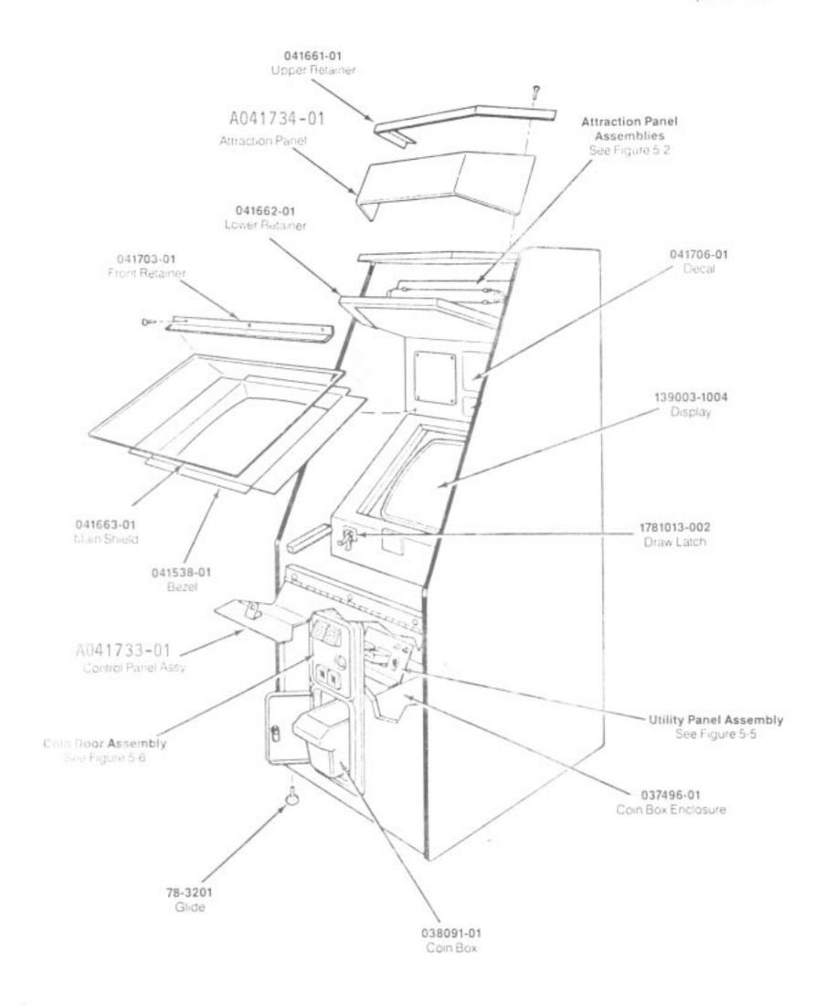
Figure 5-1 Cabinet-Mounted Assemblies A041650-01 A
