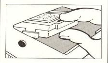
IMPORTANT: BE SURE TO HOLD THE MODULE WITH THE LABEL VISIBLE WHEN INSERTING MODULE (SEE ILLUSTRATION). FIRM PRESSURE MAY BE REQUIRED TO INSERT THE MODULE THE FIRST TIME. IF YOU HAVE PROBLEMS, REMOVE AND INSERT THE MODULE ONE OR TWO TIMES TO ENSURE THAT THE MODULE CONNECTS PROPERLY WITH THE SPEAK & SPELL LEARNING AID.
