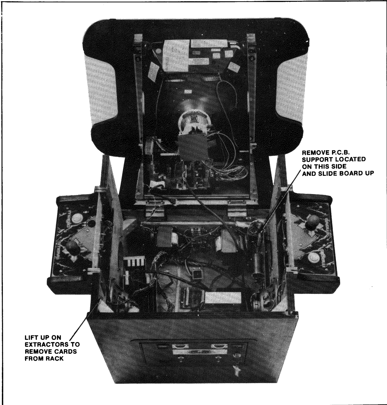
Figure 4-15 Removing Printed Circuit Boards — Cocktail
