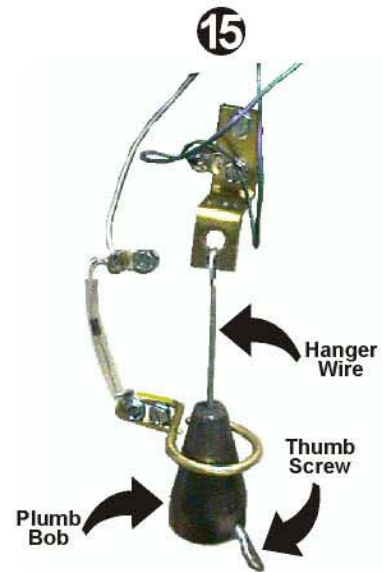
15. Install the PLUMB BOB on the Hanger Wire & tighten the Thumb Screw . Loosening the Thumb Screw & lowering or raising the PLUMB BOB makes the Games Tilt Function more or less sensitive.
