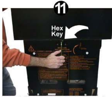
11. After the BACKBOX is in the UPRIGHT POSITION , locate the 5/16" HEX KEY . While inserted, rotate KEY with a 3/4 turn until latched & locked.
