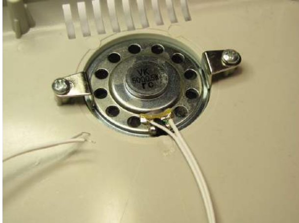
Tinned Bell wire attached to the speaker
