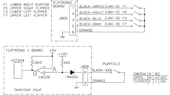
The flipper E.O.S. circuits operate similar to the dedicated switch circuit. The circuits are active low and tied to ground through the switch.
