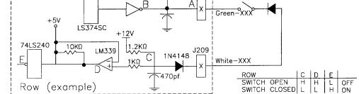
The microprocessor is constantly strobing the column side of the switch. When point "A" on the column circuit toggles low, the column side is active.
