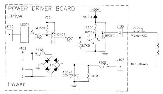
The microprocessor toggles the output of the 74LS374. When point "A" is low, point "B", the collector of the 2N5401 transistor, is high. A high at point "B" causes point "C", the collector of the TIP102 transistor and point "D", the emitter of the TIP36C transistor, to drop low. When point "D" is low, the coil is grounded through the transistor and turns on. The coil shuts off when point "A" toggles high.
