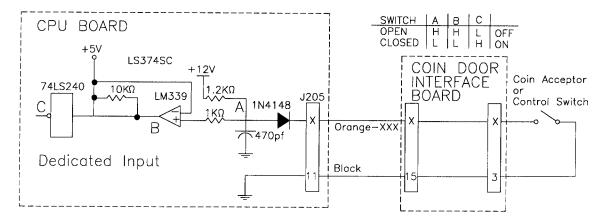
The dedicated switches operate similar in the matrix, except that instead of a column circuit there is a direct tie to ground. Therefore, the column side is constantly active (low).
