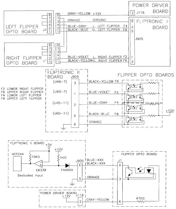
The flipper switch circuits operate similar to the dedicated switch circuit. The circuits are active low and tied to ground through the switch circuit.
