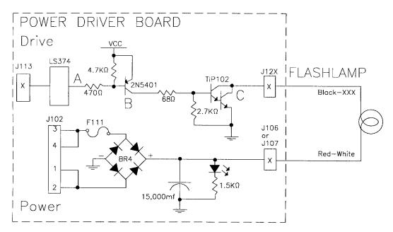
The microprocessor toggles the output of the 74LS374. When point "A" is low, point "B" the collector of the 2N5401 transistor, is high. Once point "B" is high, point "C" the collector of the TIP102 transistor is low. When point "C" is low, the flashlamp is grounded through the transistor and turns on. When point "A" toggles high, the current shuts off.
