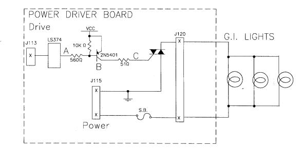
When point "A" toggles low, points, "B" and "C" are high. This turns on the triac and the desired general illumination string of lights.
