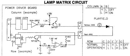
The microprocessor sends a signal to the column circuit causing the output of the UNL-2803 to toggle. When point "A" drops low, the TIP107 transistor conducts and point "B" changes to a high state. At the same time, the microprocessor drives the input of the 74LS74 low, causing a high at output "F". A high state at the base of the TIP102 causes the transistor to conducts, bringing the row circuit to ground and turning the lamp on.
