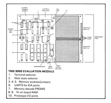
The TMS 9995 EVM may be used alone or, with an RS232 link, with a TMAM 9000 series development system. Either a telytype or RS232 terminal may be used to control the EVM. Target systems may be built up using the RAM/ROM sockets, prototyping area and prototype ports.
