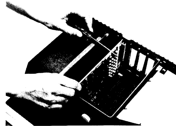
Removing a Peripheral Card
