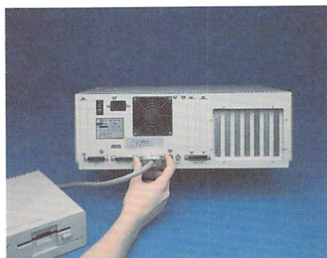
Connecting a 3 1/2-inch disk drive
